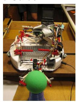
After we finished the claw and sorter we realized that it would also work for the cups with tribbles on top. When a cup was clamped and lifted the tribble would fall back like the top tribble on a tribble stack. The claw can grab the garden.
